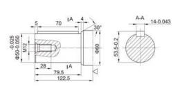
**Shaft:** cylindrical shaft, diameter 50 mm
